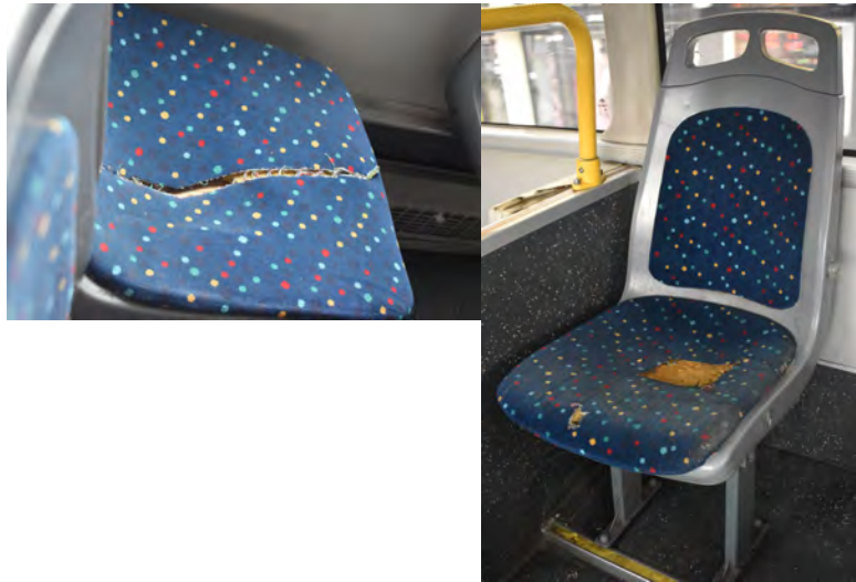
Figure 38: Deteriorated seats from the inside of a JSP bus, showing a lack of maintenance and cleanliness
