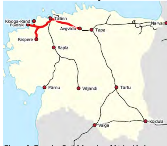
Figure 9: Estonian Rail Map circa 2016 with the electrified portions of the railway highlighted in red
